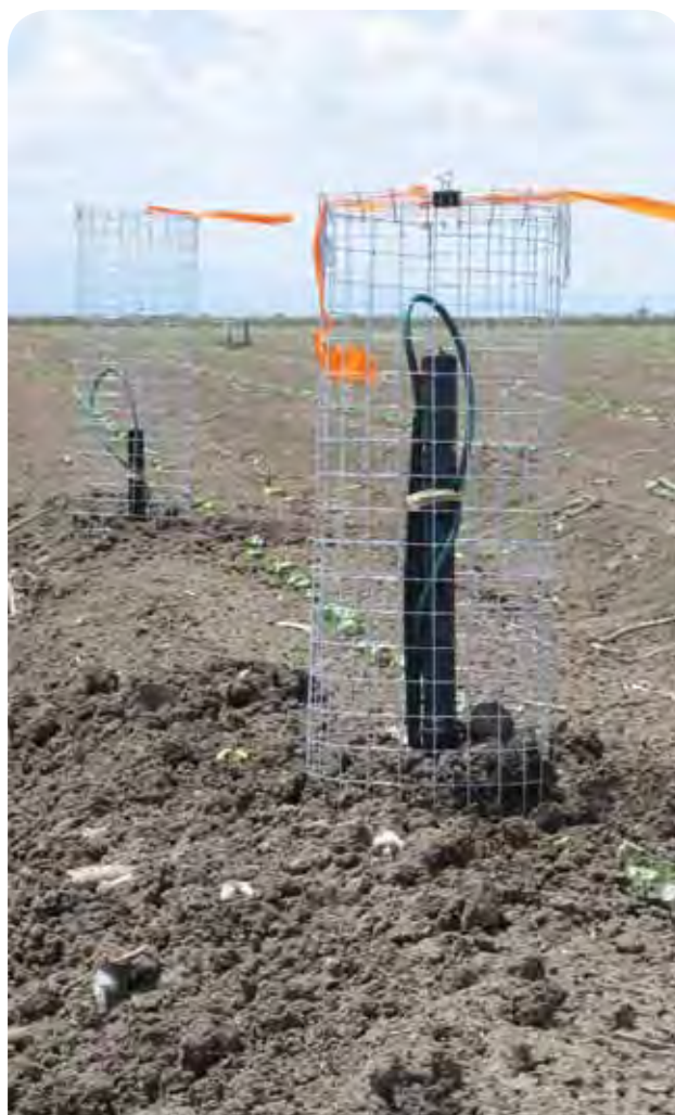
Full stops in the field installed (by Oliver Knox) to measure nitrate and ammonium in by pass irrigation water and also attempted to detect Cry proteins.
