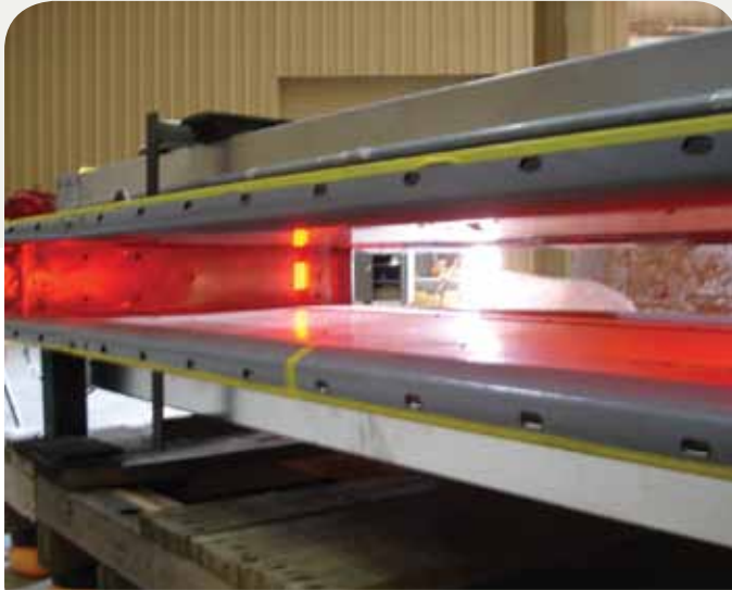
Moisture assessment and management is a fundamental problem in the ginning process. Siroduct was designed to measure the moisture of fast moving seed-cotton and/or lint during ginning. Moisture duct light sensor ready for installation
