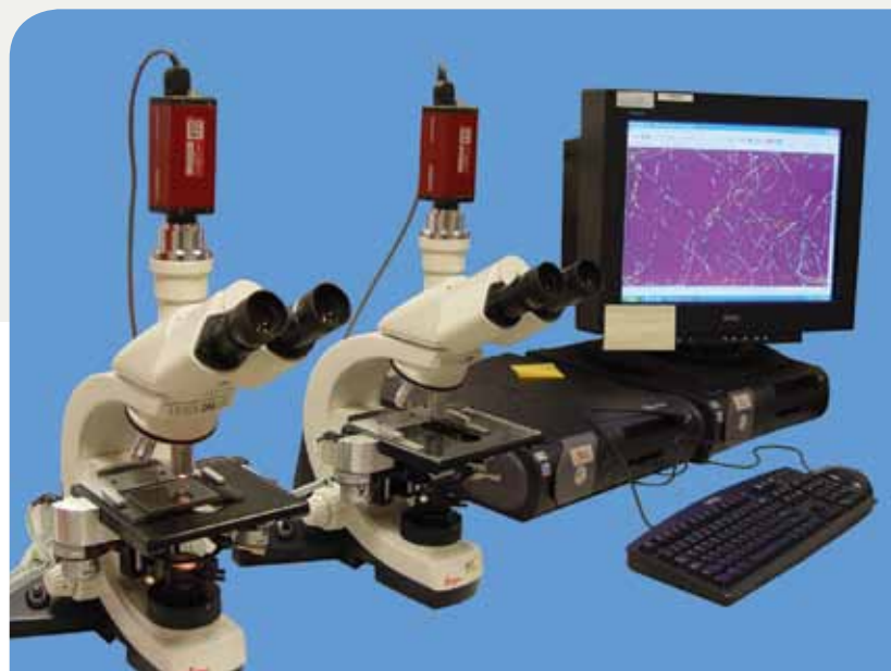
SiroMat technology centres on the use of automated polarized light microscopy to assess individual fibre samples.
