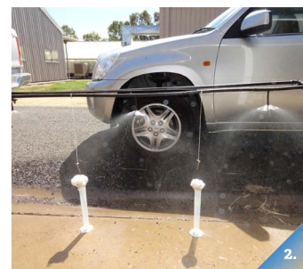
1. OVERHEAD sprinkler system used to simulate rainfall
