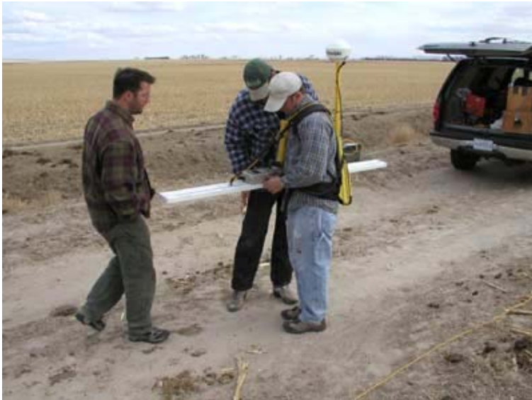
Figure 19 Eric White (USGS, OGW, Branch of Geophysics), conduct a geophysical survey in Nebraska using a Geophex GEM2 multi-frequency electromagnetic sensor.
