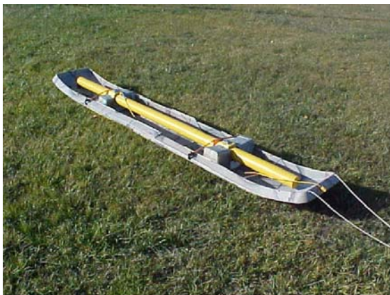
Figure 6 DualEM 2s on a rudimentary sled (Photo: John Holman, USDA-ARS)
