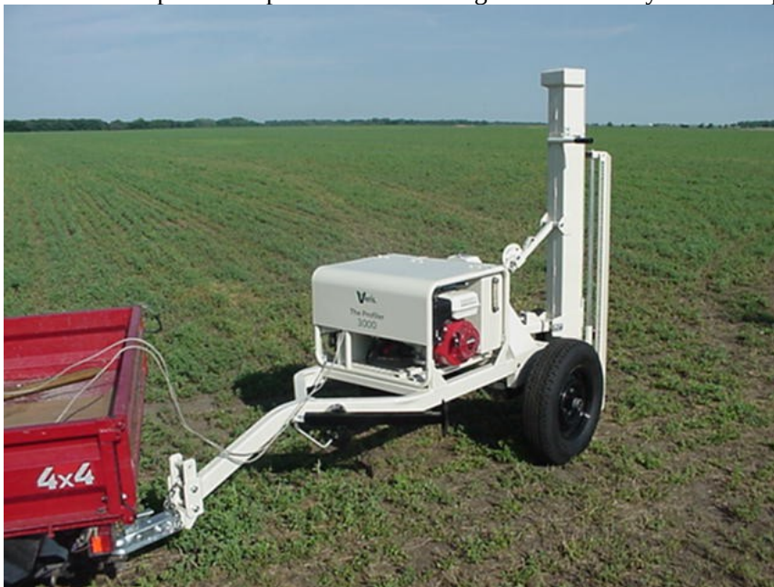
Figure 64 Veris Penetrometer with EC and pressure sensors.
