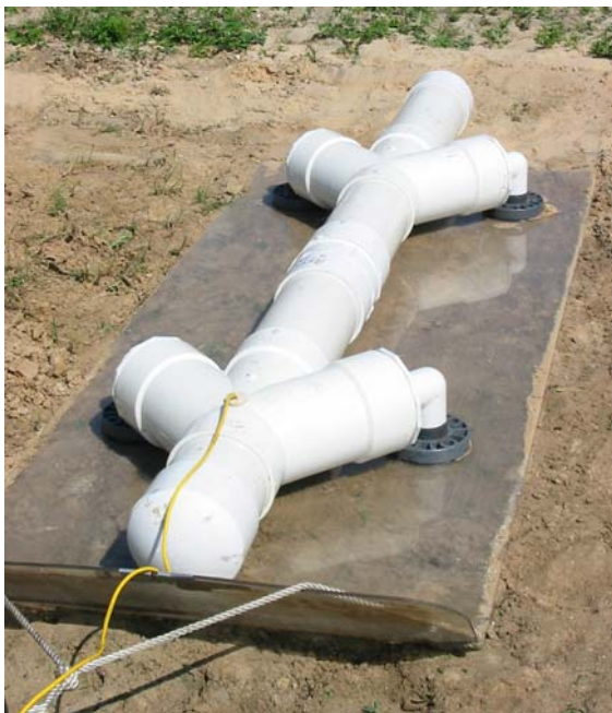
Figure 6 DualEM 2s on a rudimentary sled (Photo: John Holman, USDA-ARS)
