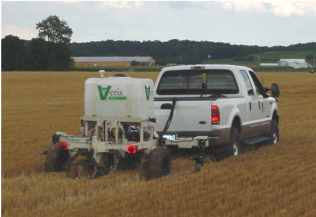
Figure 29 The Veris mobile sensor platform with electrodes sensing EC at 0.0-0.3m and 0.0 to 1.0m and pH at 0.1m depth every 12 seconds.
