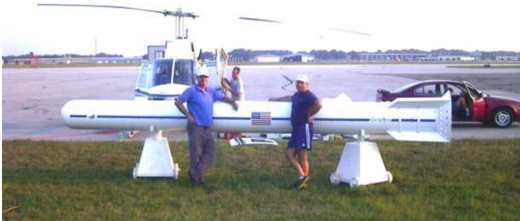
Figure 58 The GEM 2A broadband FDEM device weighing only 110 kg.
