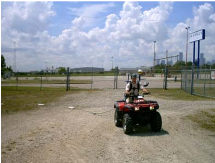
Figure 25 A capacitive coupled resistivity meter towed behind an all-terrain vehicle in Nebraska. The capacitive coupled resistivity meter (the cable and white tubes) consists of a
