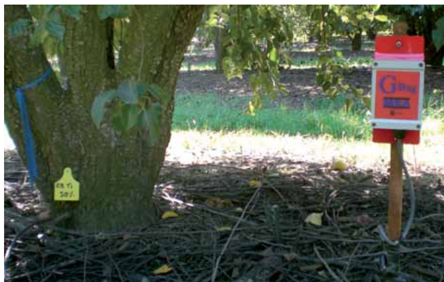
Gypsum blocks measure soil water suction.
