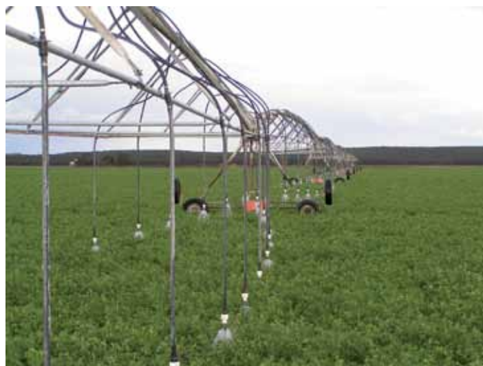
Sprinkler systems can irrigate large areas, but need water under pressure to operate.
