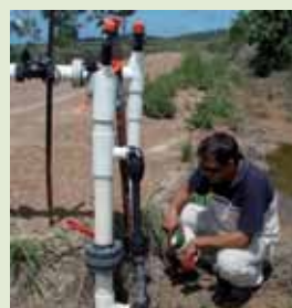
A pineapple field with randomised oxygation treatments, and (above) the venturi aeration apparatus used for oxygation.
