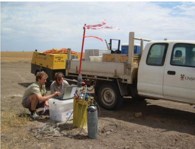
Figure 7 Slug testing monitoring bores to measure aquifer permeability.
