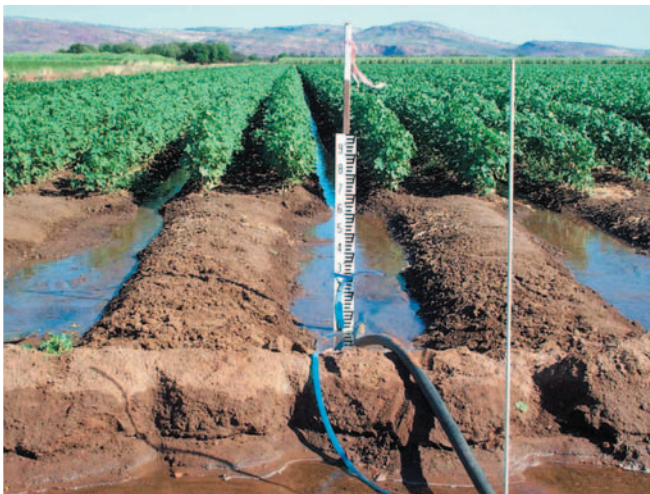
Measuring the pressure head at the siphons using a static siphon.
