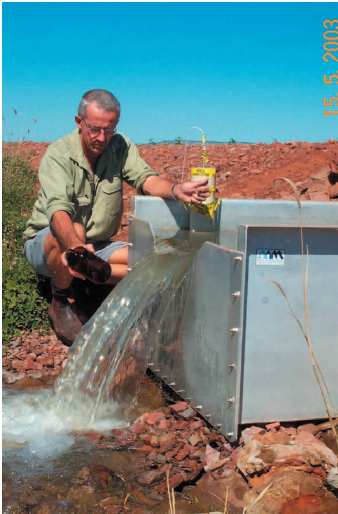
Measuring tailwater using a V-notch weir.
