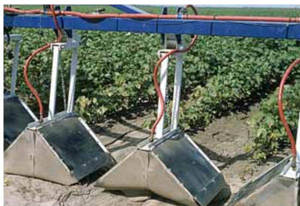
Glyphosate can be applied through spray shields to the area between the cotton rows in conventional and Roundup Ready cotton varieties. The spray shields prevent the herbicide contacting the foliage of the crop.
