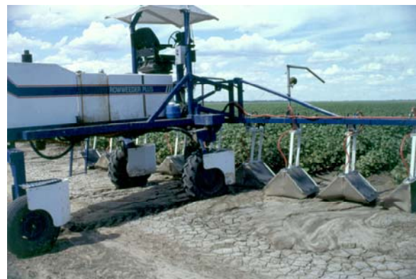
A purpose-built, high clearance sprayer set up for shielded spraying.
