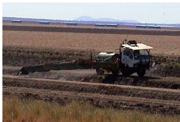
A purpose-built sprayer, designed for spraying irrigation channels. Photo by Sandra Williams.
