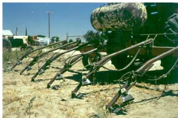
A homemade flame weeder for controlling weeds in the inter-row area.
