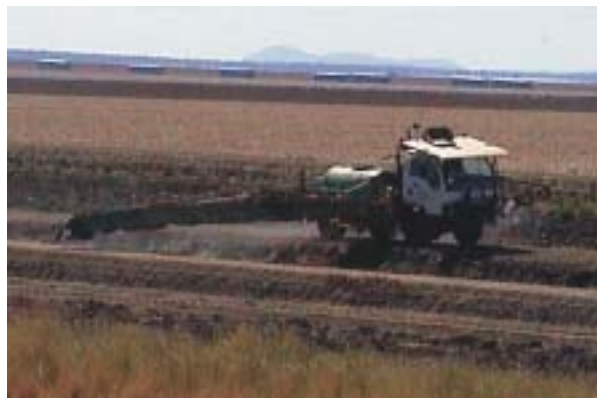
A purpose-built sprayer, designed for spraying irrigation channels. Photo by Sandra Deutscher.
