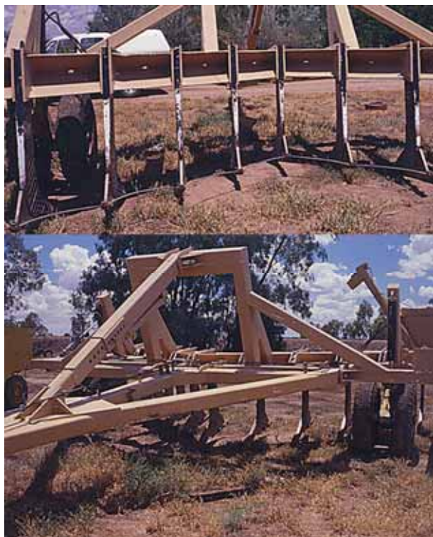
A trailing ripper set up for heavy cultivation of nutgrass after picking. Note the steel cable across the rippers (top photo) designed to cut the nutgrass roots during ripping.
