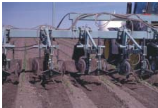
Inter-row cultivation rig set up for one-pass cultivation and cold-flow nitrogen application.
