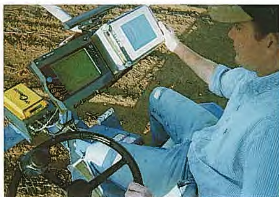
Figure 1a. Trimble Ag132, GPS400, RMD and 486 data logger/control box.
