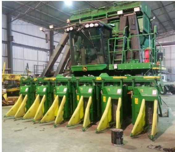
Figure 4. Round bale pickers are progressively replacing aging traditional basket pickers
