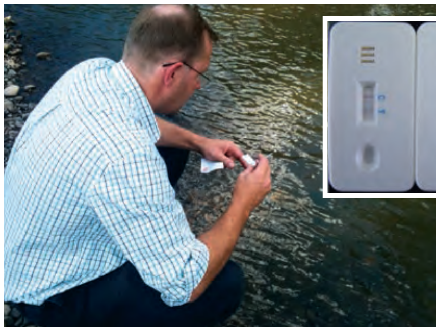
AT LEFT: Quick Test is a breakthrough in environmental analysis of water resources and (inset) a Quick Test example showing Diuron levels.
