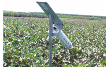
Figure 1: Infrared canopy temperature sensor installed in a cotton field
