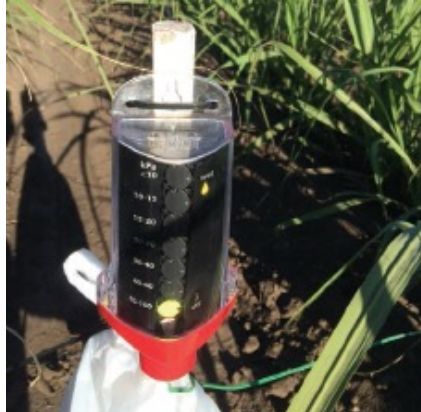
G-Dot indicating that the kPa of the soil where it is installed has reached the 60–100 kPa reading.
