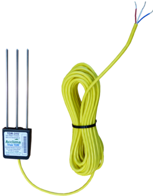
Figure 1: Acclima TDR sensor with 150 mm long sensing rods and ten metres of cable for connection to SDI-12 capable datalogger (Acclima, 2017)
