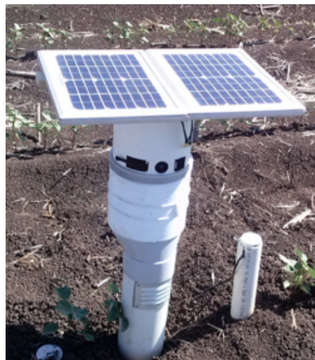
Vertical installation of MP406 sensors installed at three depths with access tube
