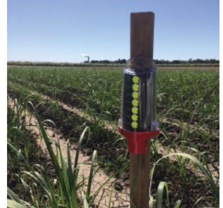
G-Dot indicating soil profile has reached full point or saturation as indicated by the readings of less than 10 kPa
