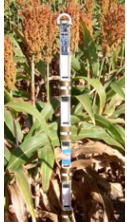
Figure 1 : The inner components of a capacitance probe lifted from its buried plastic pipe sheath, showing the logger board on top, and the five pairs of cylindrical gold coloured electrode plates (sensors) used at five different depths in the soil.
