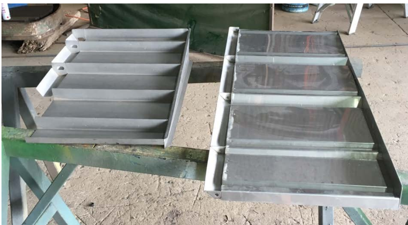
Plate 1: Models fabricated by the Commins brothers to describe the irrigation layouts, furrow along bays (LHS) and furrows across bays with rollover banks (RHS).
