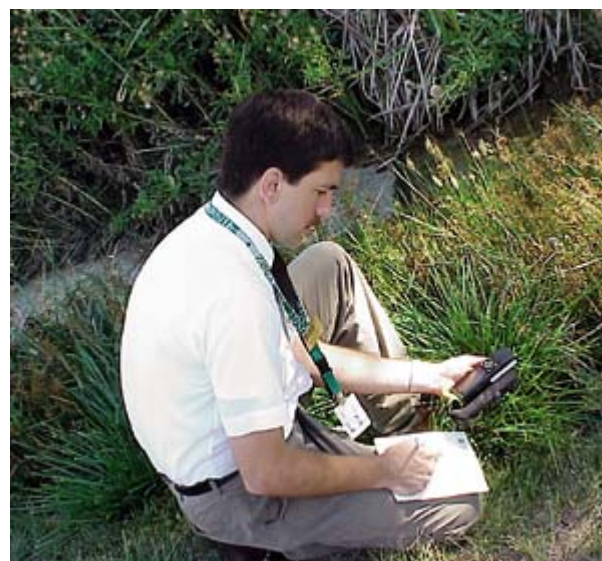
Figure 3-16 Collecting latitude and longitude coordinates with a global positioning system (GPS) receiver
