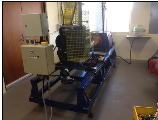
Figure 80. HATZ apparatus with a Diesel/Gas LPG injection system installed.
