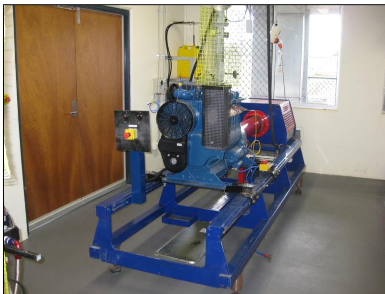
Figure 68. HATZ engine and dynamometer testing apparatus, USQ, 2014.
