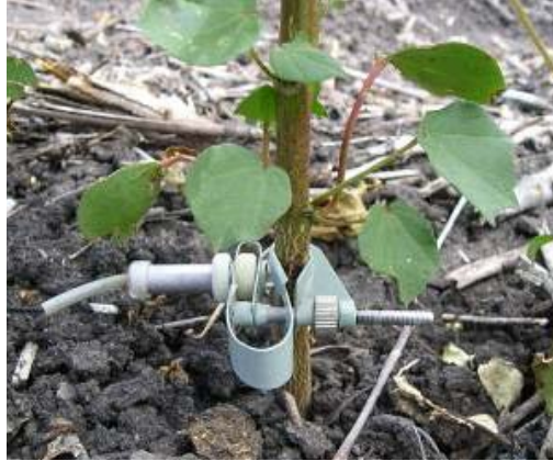
Figure 2.7: Dendrometer measuring stem diameter fluctuations
