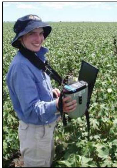
Figure 3.1: Handheld multispectral scanner with computer logging in front harness
