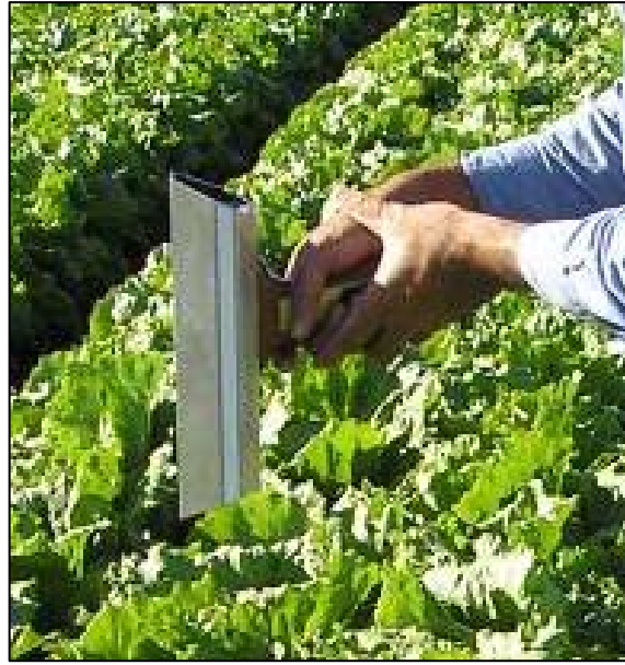
Figure 3.6: Using a handheld infrared thermometer to measure canopy temperatures
