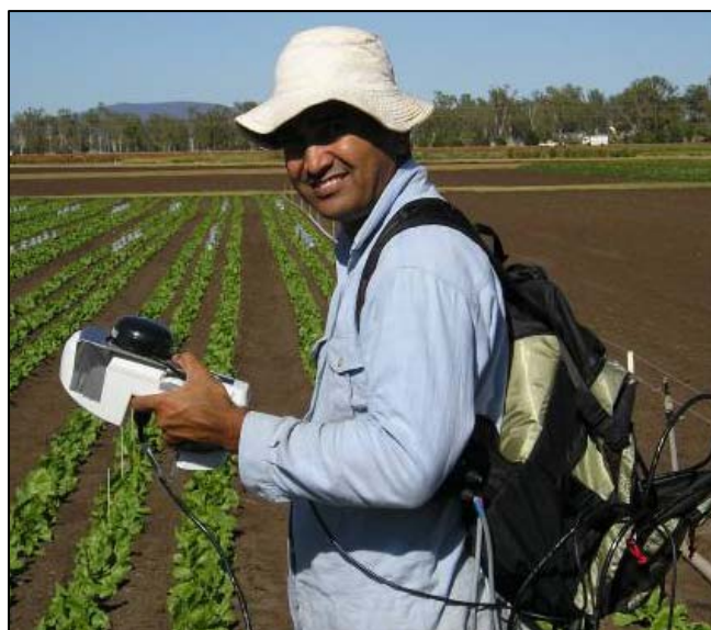
Figure 3.2: NDVI Greenseeker sensor with logger in backpack.
