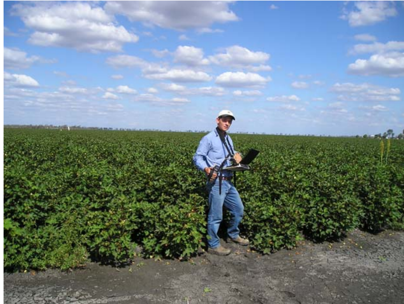
Figure 3. ASD FieldSpec Handheld radiometer used to measure crop canopy reflectance prior to leaf water potential measures.
