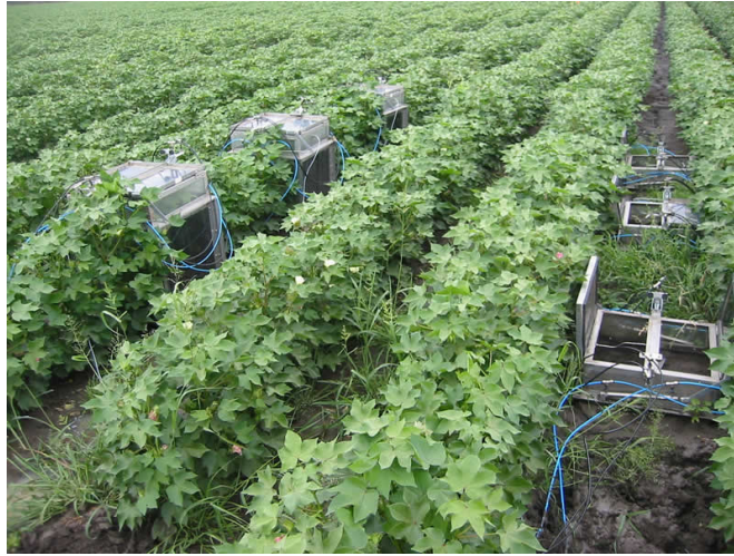
Figure 2. Gas sampling chambers (with and without 50 cm extensions) used at Dalby, Queensland for greenhouse gas emission experiment during the 2005/06 season.
