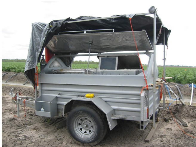
Figure 1. Trailer based greenhouse gas sampling and analysis unit.
