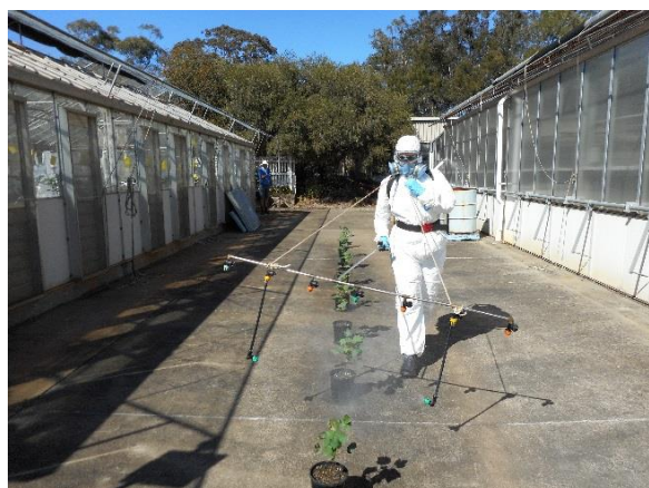
Hand-held spray boom used to treat experimental plants
