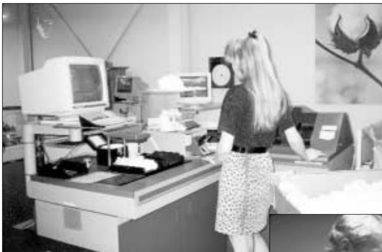
Left: Cotton classing using the latest High Volume Instrument (HVI) system.
