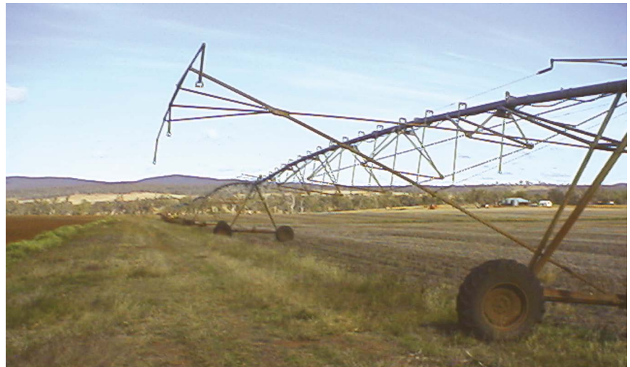
Figure 5.5.12. Field test results showing three times the normal amount of water being applied around the tower through interception of sprinkler water by tower structure
