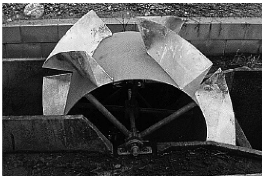
Figure 1.7.8. – Dethridge-Long meter showing the elongated vanes (Sunwater)
