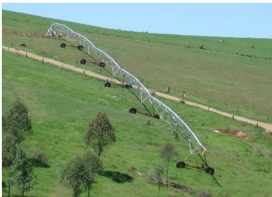
Figure 5.1.10. Centre Pivot irrigation system (Photo: E. Parr)
