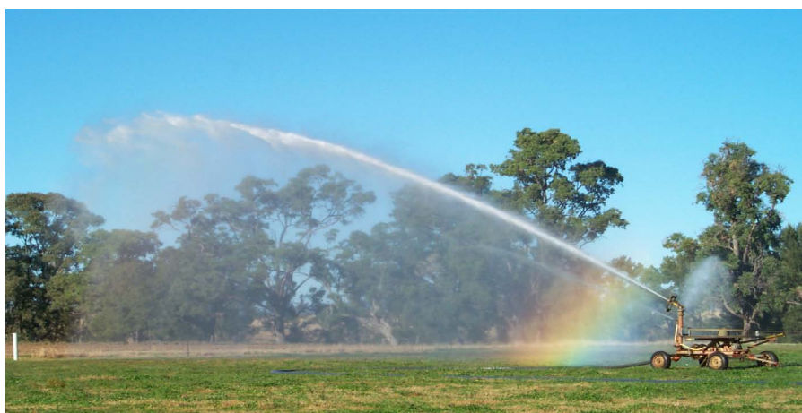
Figure 5.1.8. 'Big-gun' Travelling irrigator
