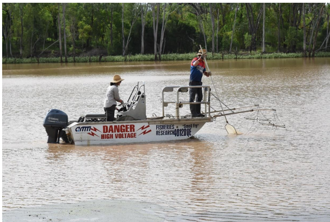
Figure 5: Electrofishing boat in operation on the Mackenzie River.
