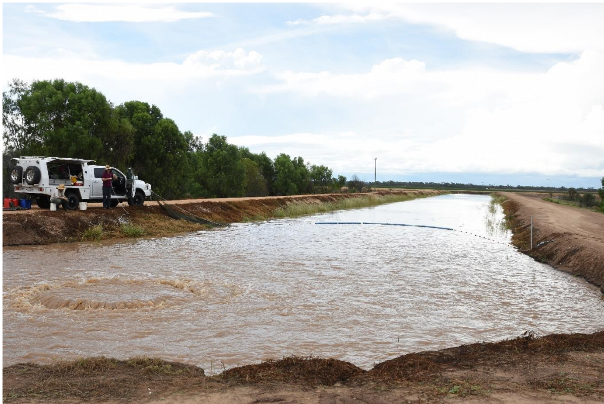
Figure 4: Outlet sampling net in place. Note the float line and extra floatation from pool noodles across the centre of the net.
