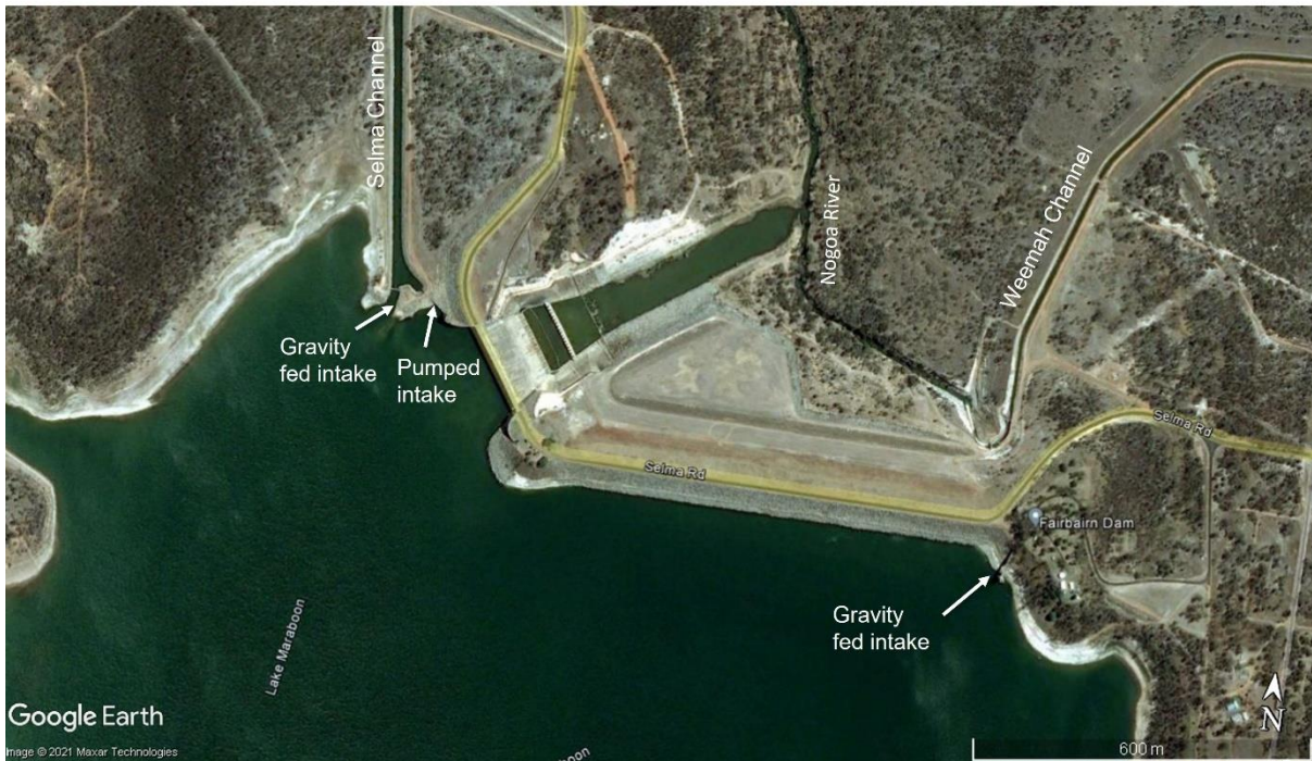
Figure 3: Satellite image showing intakes for diversion channels from Fairbairn Dam. Selma Channel intake (upper left) when gravity fed, or when pumped into the channel at dam levels below 68% capacity. Alternatively, water passes from the intake (lower right) through the bottom of the dam wall to be released into either the Nogoia River, or the Weemah Channel.
