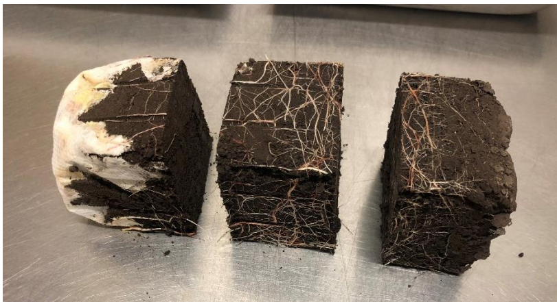
Figure 1. Soil core cut into three equal sections (top, middle, and bottom) to assess the vertical movement of the reniform nematode. Soil and root subsample in each section was analysed separately to quantify the reniform nematodes.
