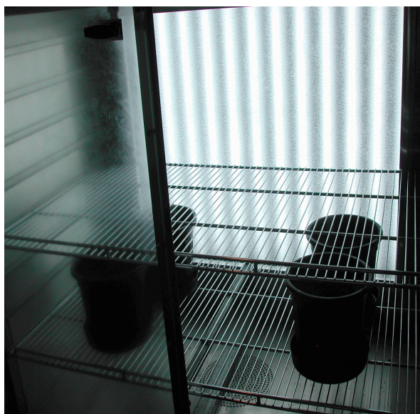
Figure 3. The internal arrangement of the 750L plant growth cabinets showing the variable shelf positions and light arrangements
