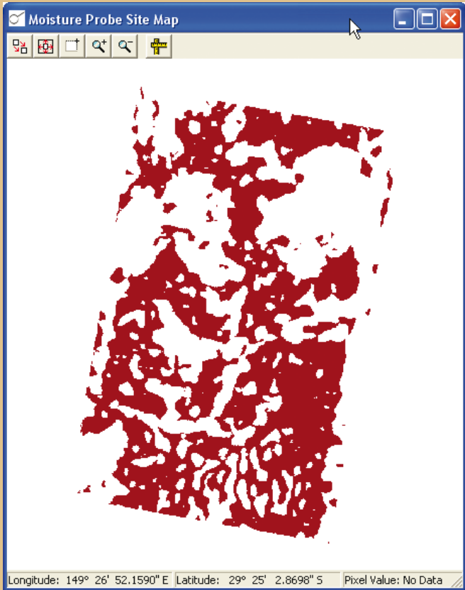
FIGURE 4: Final map which best represents majority soil type, closest to majority slope and in some cases removal of areas of high previous cut.
