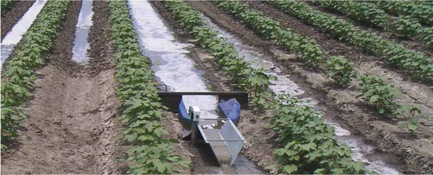
Using flume meters to measure water flow rates.
