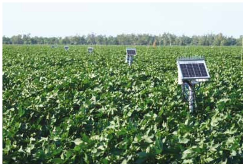
Soil moisture probes monitoring different irrigation treatments.
