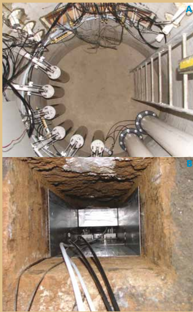
FIGURE 1: The ACRI lysimeter facility. A: View looking down into the access shaft, showing the window through which the collection trays are installed (top) and the six collection tanks into which the drainage passes for measurement (left and bottom). B: one of six collection trays during installation, showing the horizontal tunnel, drainage and vacuum tubes and space for a second tray in front. Two other pairs of trays were later installed either side of the tunnel shown.
