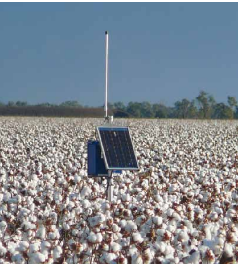
Soil moisture probes are used to monitor moisture throughout the season. The cotton industry has the highest adoption of soil moisture monitoring tools compared to other crops.
