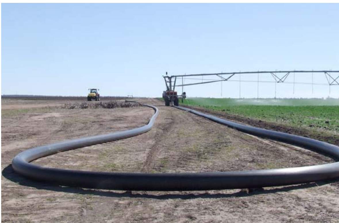
A hose-fed lateral move system.
