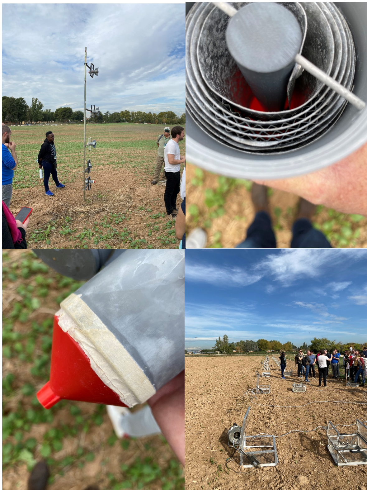
Figure 3. Measuring ammonia losses at the “La Chimenea” field station using the gold standard “Integrated Horizontal Flux” method. The shuttles are placed at standardised heights of 0.25, 0.50, 1.0, 1.5 and 2.75 m above the soil surface. The plots are circular (20 m radius) and measuring ammonia from Urea and Urea+ inhibitor applied plots. The ammonia is captured in the shuttles on the stainless-steel spiral coated in oxalic acid. It is then extracted from the stainless-steel spiral using deionised water. Bottom right - the GHG chambers in another field capturing nitrous oxide emissions under cultivation and min-till rotation experiments.
