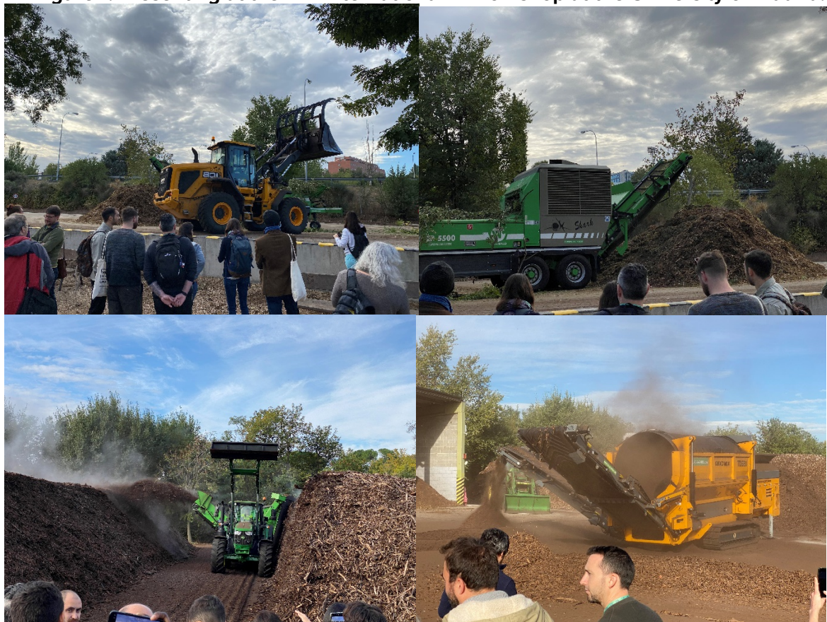
Figure 2. Circular economy tour – Madrid city park plant residues from pruning are processed at the “Migas Calientes” Composting facility. The composted residues are then trucked back to the garden beds in the city.
