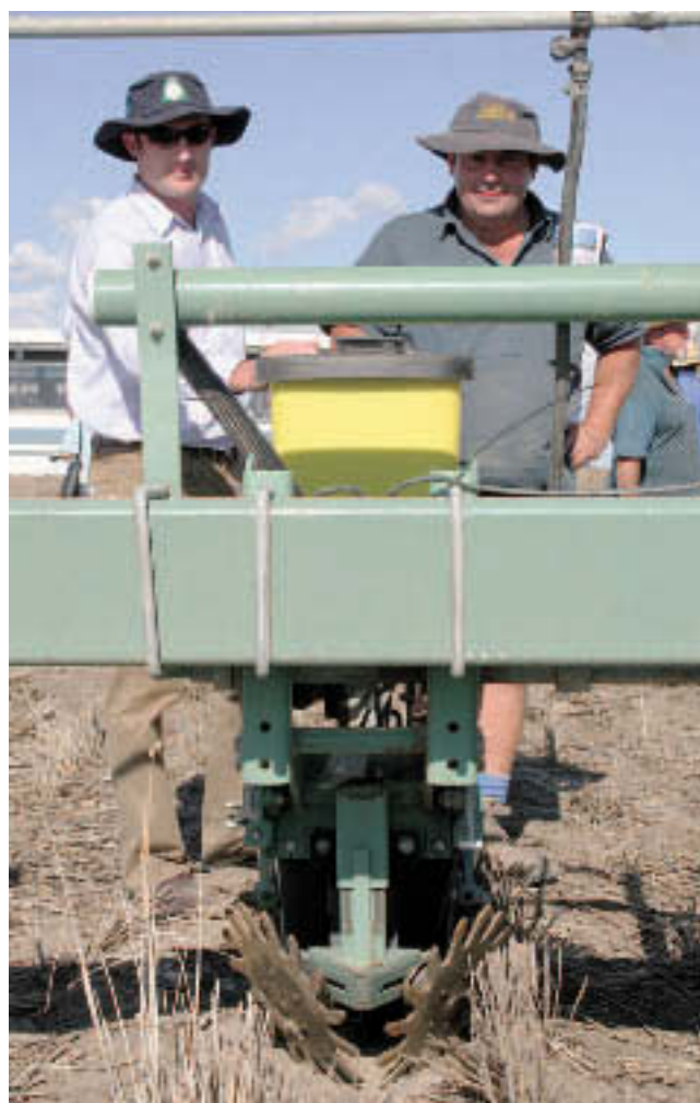
PJ Gileppa of Auscott Narrabri and Wee Waa grower Charlie Arnott have a closer look at the planter which has been modified to plant cotton between rows of standing cereal stubble.
