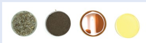
The stages in processing cotton gin trash to ethanol: raw trash; 'pretreated' or cooked trash; extracted sugars; and the fermentation beer (sugars to ethanol).
