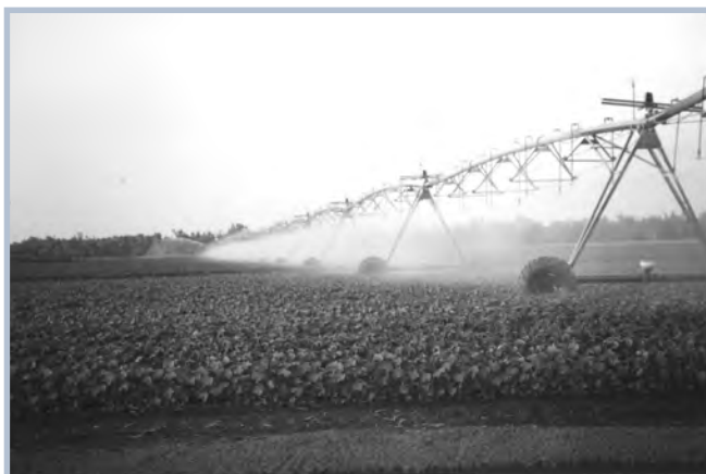
Figure 26: Lateral move machines are among alternative water delivery methods attracting more interest
