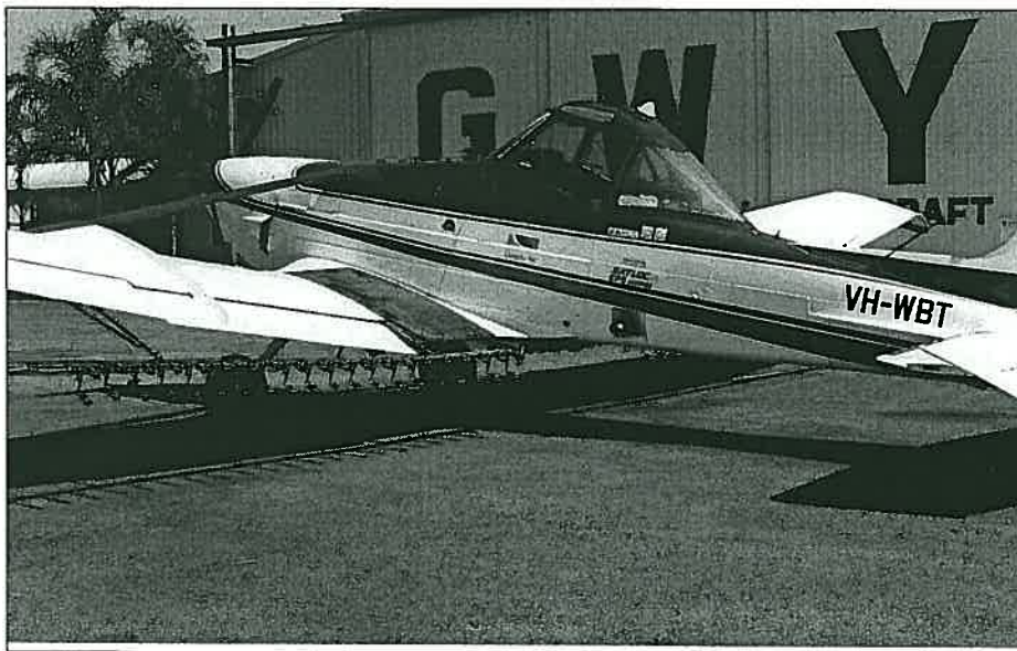
The aircraft fitted with the 80 spectrum electrostatic nozzles prior to the trial.
