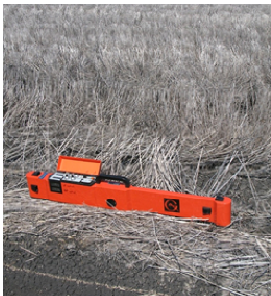
Figure 1. EM38-MkII in the field. The unit is sitting in the vertical dipole position. Horizontal dipole is obtained by placing the unit on its side.
