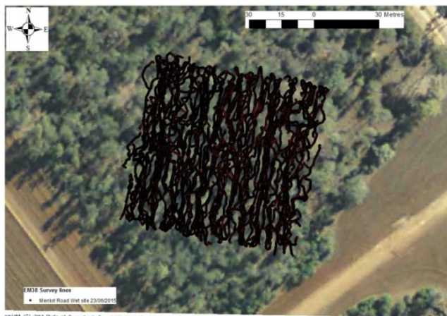
Figure 4. EM38 1 m interval survey conducted at Merriot road wet site.
