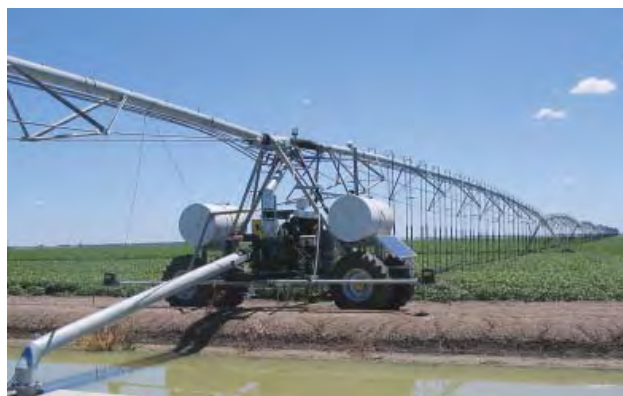
Overhead irrigation systems such as this lateral move are increasingly water use-efficient and cost effective
