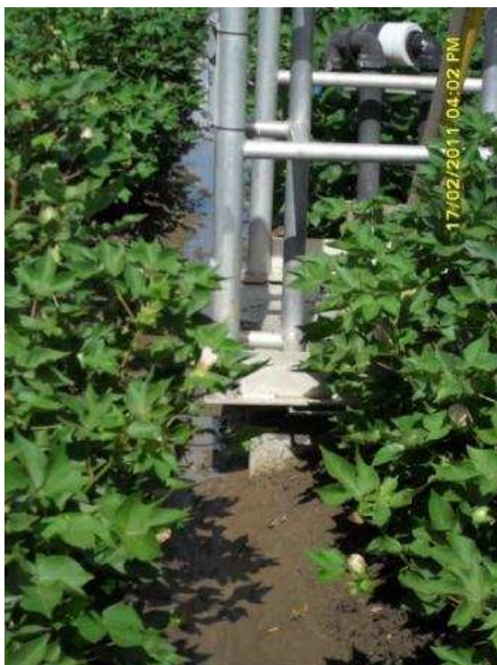
Fig. 44. Ponding of water near lysimeter
