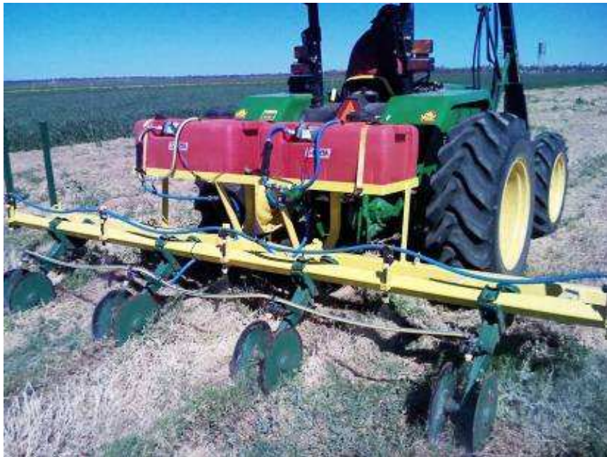
Fig. 4. Final design (“Stage 3”) of mulching implement
