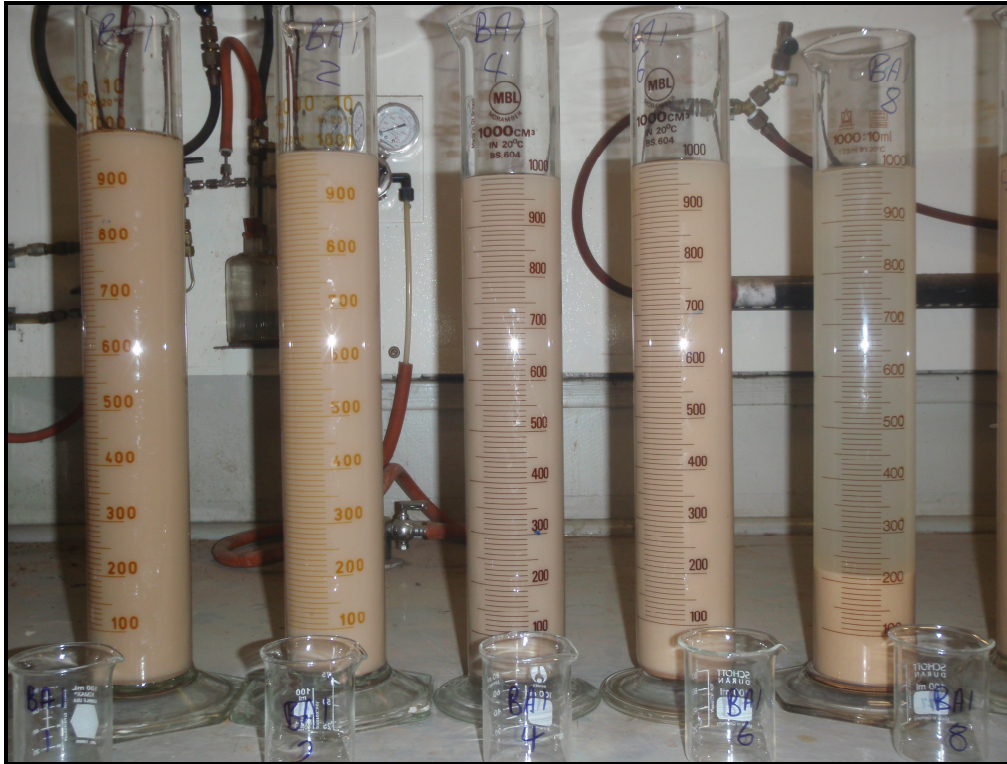
Figure 3.8. The measuring cylinder on the right contains Mount View (600-800 mm depth) soil for particle size analysis that was observed to flocculate after approximately 2 h, as a result of naturally occurring gypsum (1.35% total gypsum, Table 3.5)
