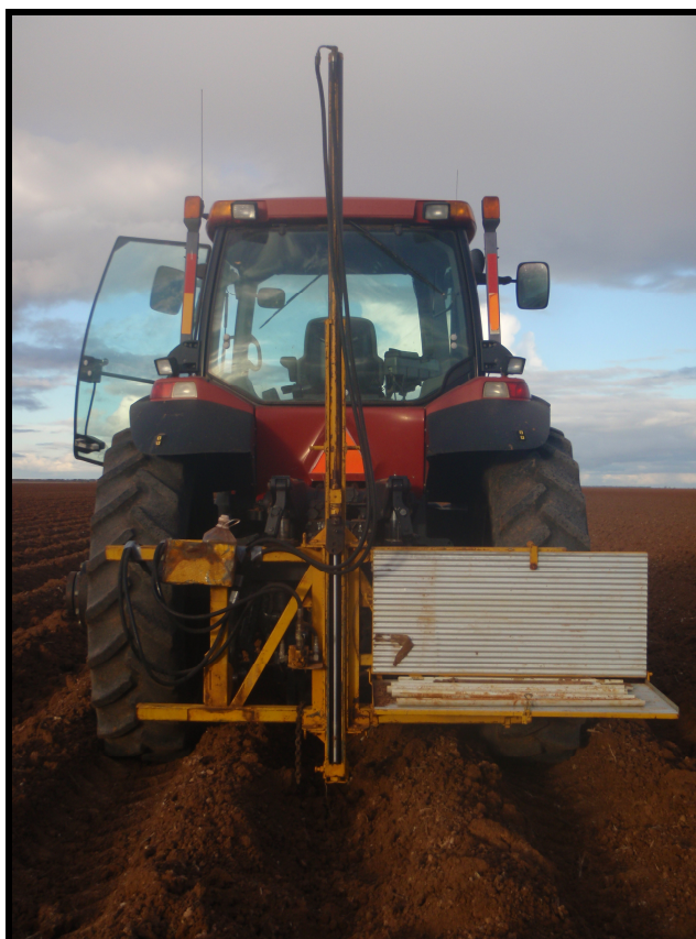
Figure 3.7. Single-stroke tractor-mounted hydraulic corer used for soil core sampling after 2.5 years
