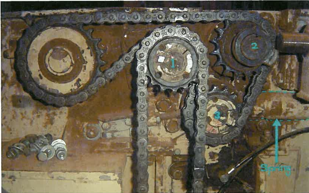
Figure 3 – Photo showing proposed location of calibrated spring to the feed roller (3).
