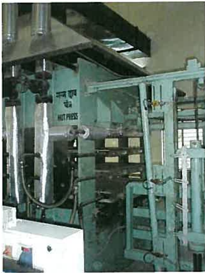
Figure: The hot press used in the manufacture of particle board from cotton stalks.
