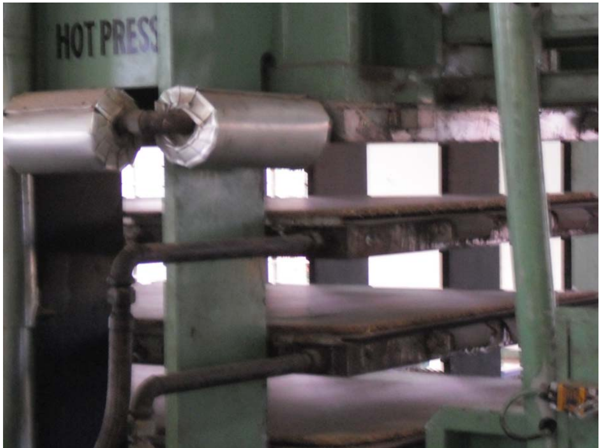
Figure 5. Particle board manufacturing from cotton stalks at GTC, Amravati Road, Nagpur.
