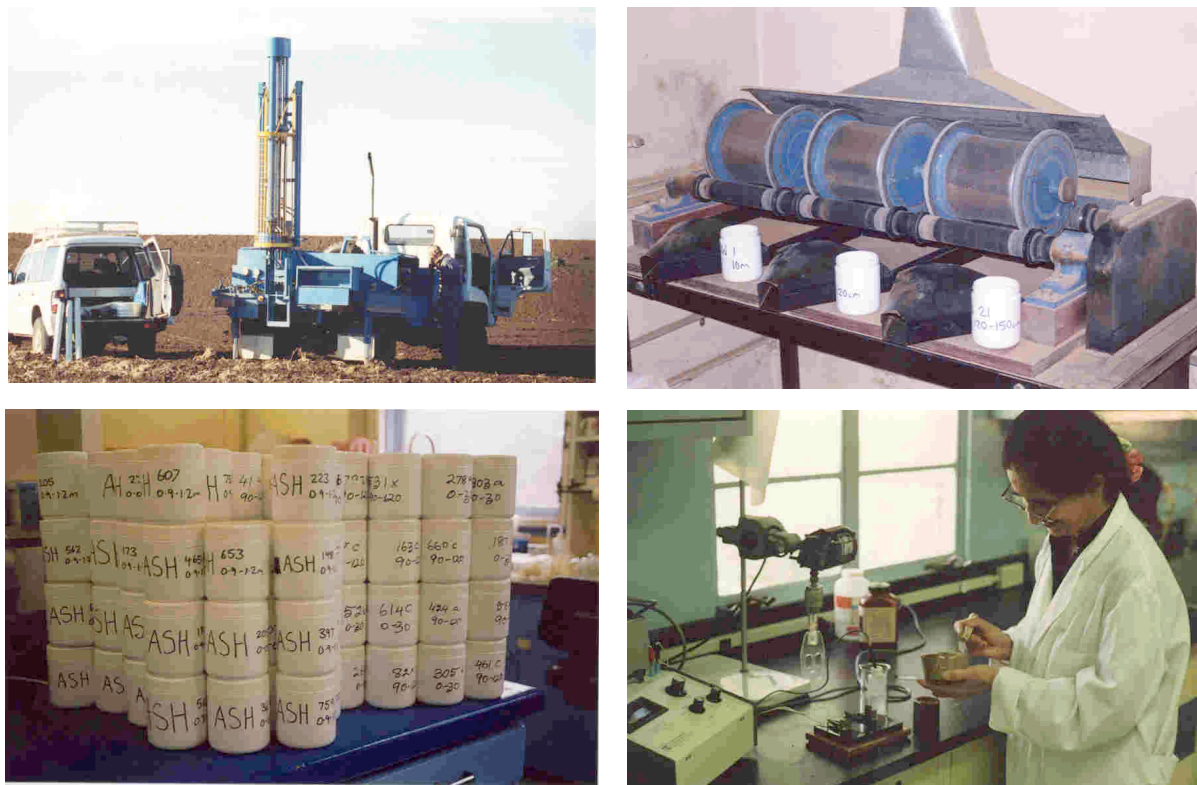
Figure 5. Soil data collection involved a) sampling to depths of 0-2...15 m), b) soil drying and grinding, c) soil storage and d) laboratory analysis (i.e. EC_e -dS/m, particle size fractions, exchangeable cations, pH, chloride content, etc.).
