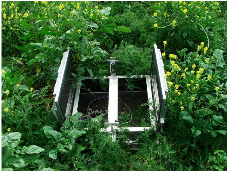
Figure 8. The vegetation cover and the measurement chamber in the fallow cropping sequence of field 6, ACRI. The vegetation inside the chamber was manually removed to measure the soil respiration and typical fallow periods are devoid of vegetation.
