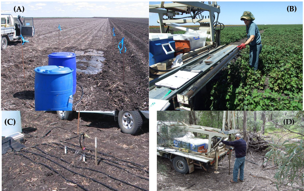
Figure 4 (a) Wetting up and (b) sampling soil for drained upper limit and bulk density, (c) tensiometers used to check matric potential of the subsoil, (d) sampling in native vegetation.
