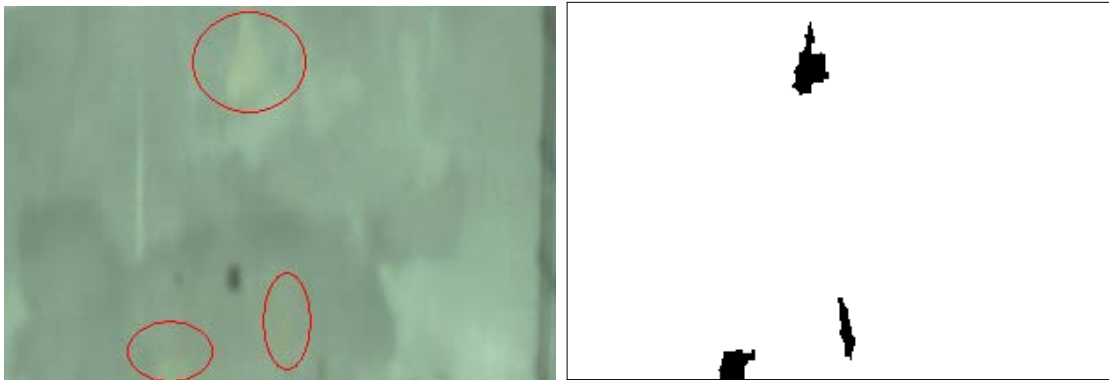
Figure 33 (a) – Detection of pale yellow contaminant – setup 1
