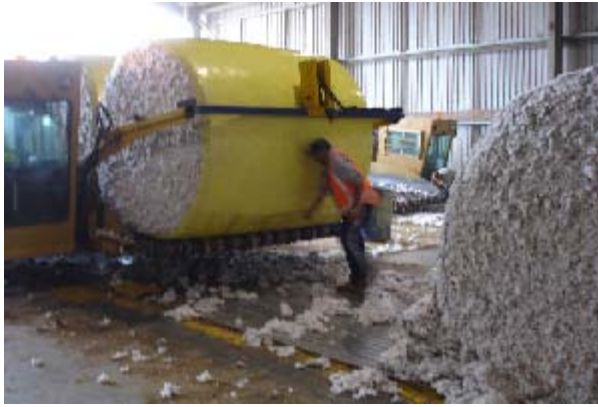
Figure 2(b) – Removing round module wrap in the module bay of a gin
