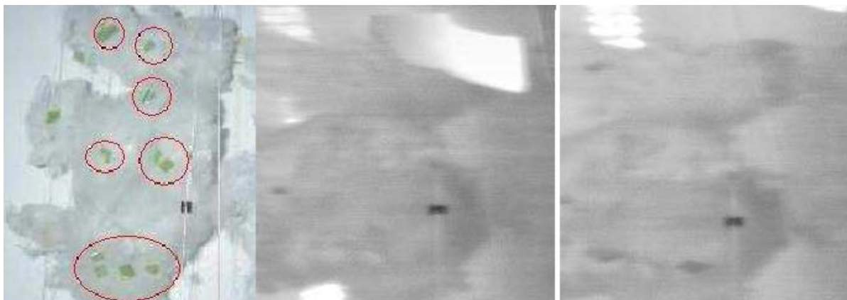
Figure 19(a) – Yellow plastic contaminant in cotton by visible light and (b) and (c) the same fov illuminated by two levels of UV light intensity
