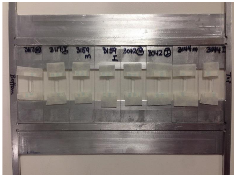
Figure 8 – Mounting frame for SAXS/WAX beamline being loaded with slides containing an array of aligned single fibres side-by-side.
