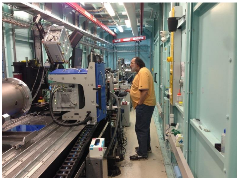
Figure 10 – Scale of the AS SAXS/WAX beamline and hutch. Dr Jeff Church examining the specimen frame position before measurement.
