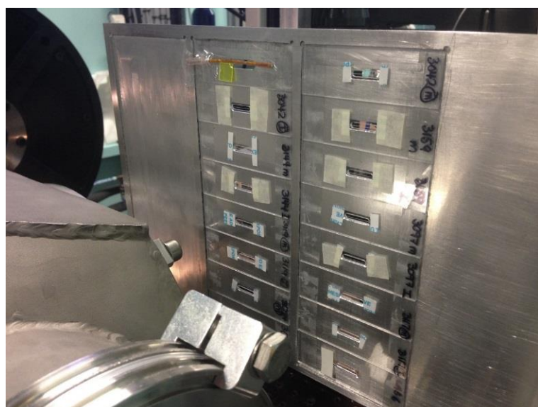
Figure 9 – Mounting frame in position in front of WAX detector. A stepper motor and camera is used to guide frame into position of the beam. Orange tube in top LH corner contains X-ray crystal standard.
