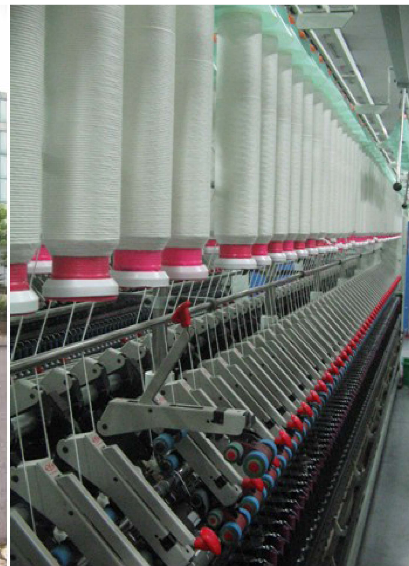
Spinning frame showing the spinning of high quality fine count yarn in the Chongqing Sanxia Mill
