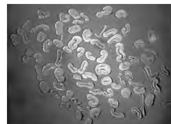
The cross section of a cotton yarn showing the packing and interaction of individual fibres. In this yarn cross-section seventy eight individual fibres are distinguishable. Changes in micronaire affect how many fibres make up the cross section of the yarn affecting its strength. (Photo: CSIRO)
