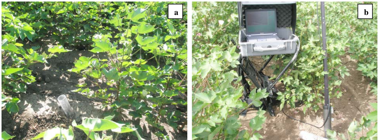
Figure 4(a) Clear plastic minirhizotron access tube, installed 30° from the vertical (b) collecting data using the minirhizotron
