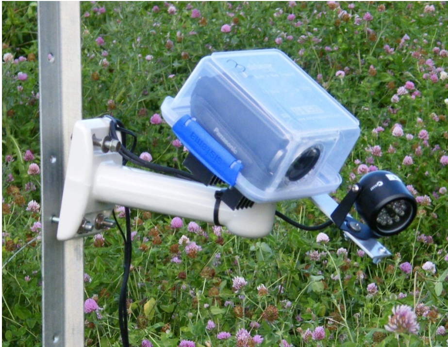
Figure 2: Camera unit with humidity cover set up in a pasture of clover. A Perspex window provides a clear section for the camera to record through.
