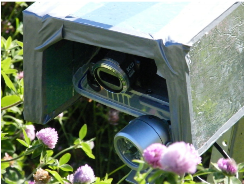
Figure 5: Details of camera under the sun shield, note that the humidity cover is not present in this picture. The Perspex window reduces the quality of the picture so when conditions are dry we used the cameras without their humidity covers.
