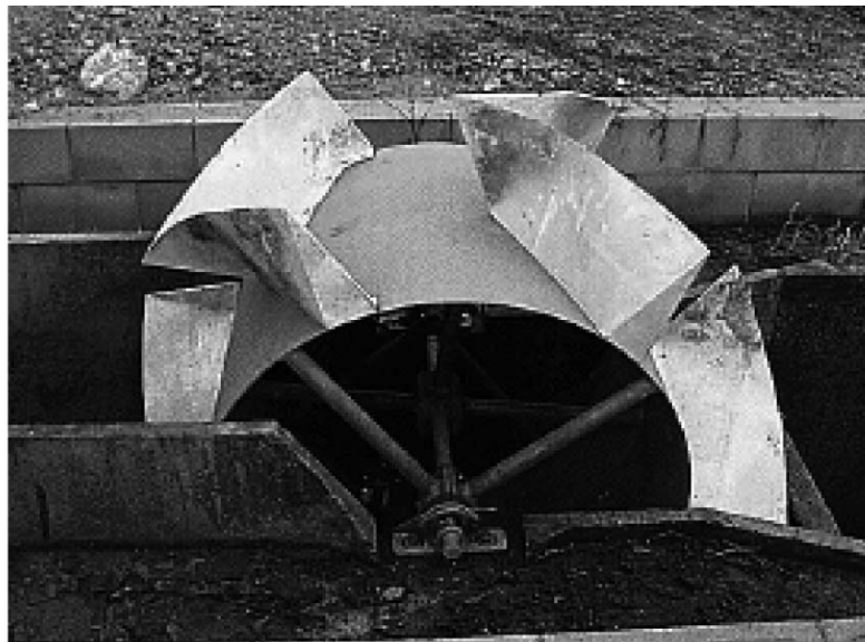
Figure 8 – Dethridge-Long meter showing the elongated vanes (Sunwater)
