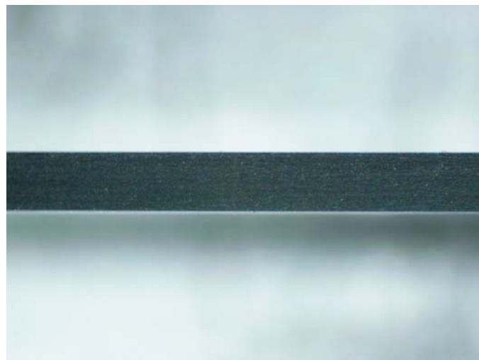
Figure 13 - Optical micrograph showing surface of edge of specimen 11 after polishing (specimen thickness is 0.9 mm).
