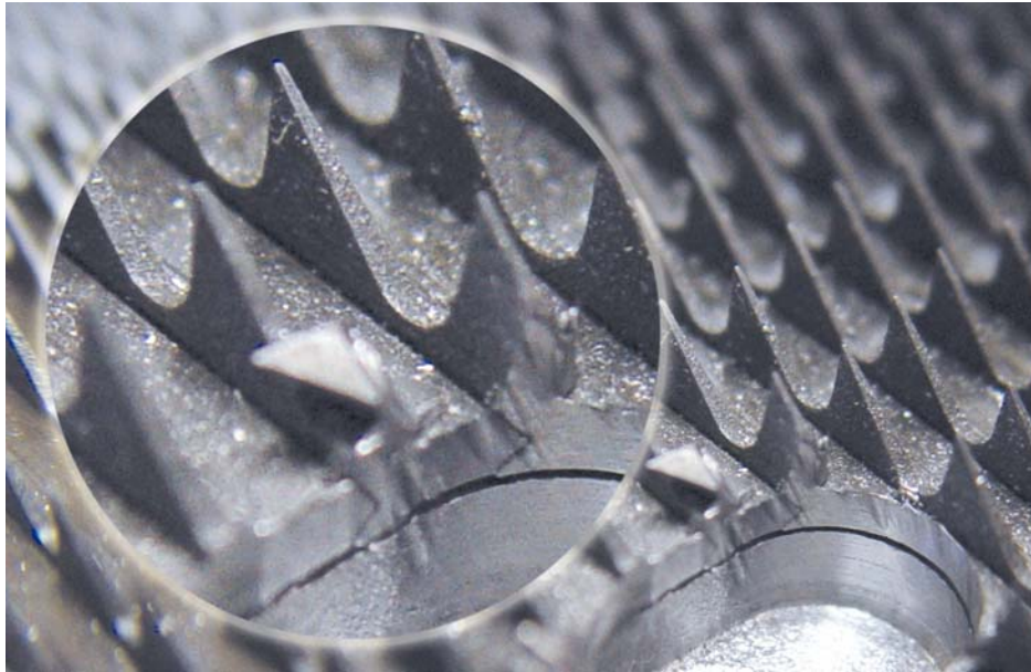
Figure 2 shows a cross sectional magnified view of the inter-locking mechanism of the wire wound onto the saw cylinder.
