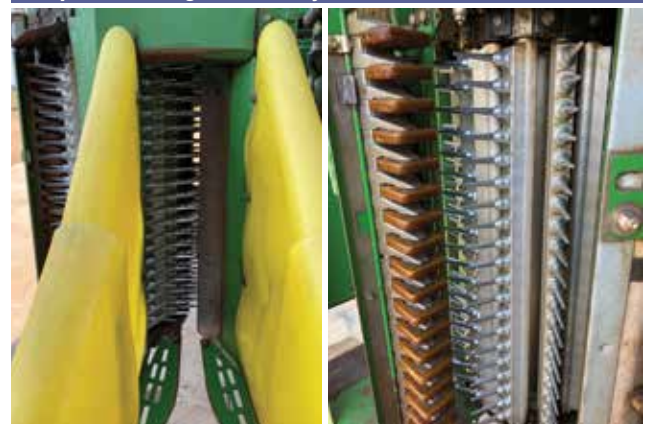
FIGURE 1: Spindle pickers require regular maintenance to operate at high efficiency.
