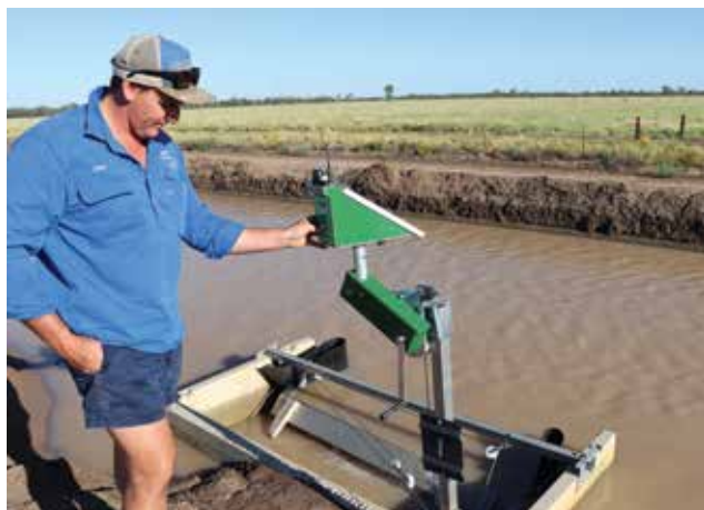
St George grower Lucas Wuersching checks over irrigation equipment being used to automate a bankless channel (tailwater backwater) system, with a range of on-farm sensors connected over a LoRaWAN network on the farm. To listen to a podcast with Lucas and Craig Saunders discussing the system, scan the QR code (below).
