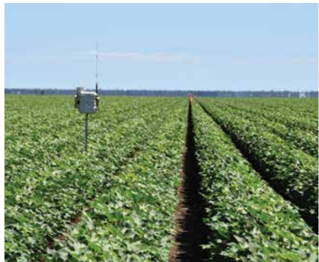
Monitoring soil moisture and irrigation performance helps schedule irrigations. (Photo: Lou Gall GVIA)
