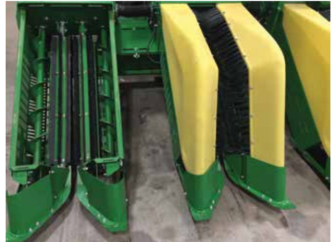
The stripper uses brushes and bats to strip seed cotton from bolls. (Photo: René van der Sluijs)
